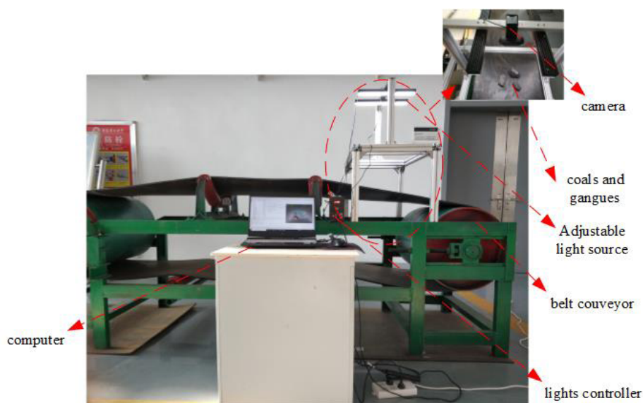
Fig. 7. Coal and gangue identification and location device
